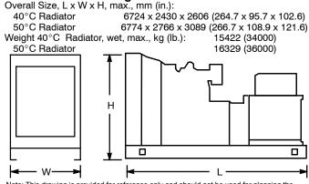
Note: This drawing is provided for reference only and should not be used for planning the installation. Contact your local distributor for more detailed information.
