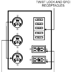
CS-6369 TWIST-LOCK RECEPTACLES (3) 240/139V, 50 AMPS GFCI RECEPTACLES (2) 120 VAC, 20 AMP
