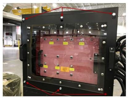
Note: There is a safety disconnect switch which will shut down the unit once you remove this back-alternator panel.
