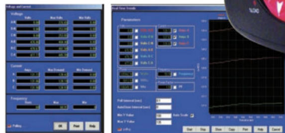
Avtron ADMS Digital Meter, Real-Time Data Logging and Trending Screens.
