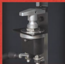
Lock. Battery Disconnect
