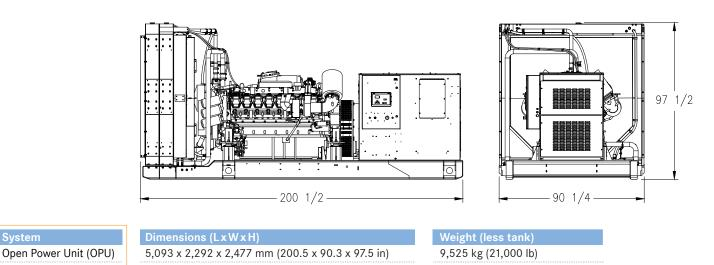
Weights and dimensions are based on open power units and are estimates only. Consult the factory for accurate weights and dimensions for your specific generator set.
