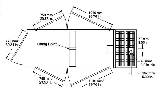
Generator can be placed on MQ Power Trailers TRLR75XF, TRLR85XF, and TRLR125XF.
